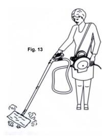
IMPORTANT: When using the steam cleaner with the shoulder strap, avoid rocking or tilting the unit excessively as this may cause water to enter the hose and be discharged along with the steam.
